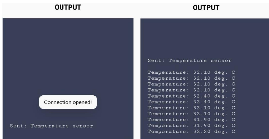
Figure 6: Temperature readings (from DHT11 sensor) being printed on output window
